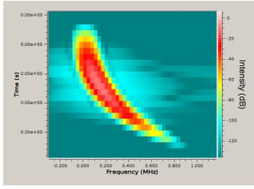
**Figure 1: The frequency and time domains of an exponential chirp.**
