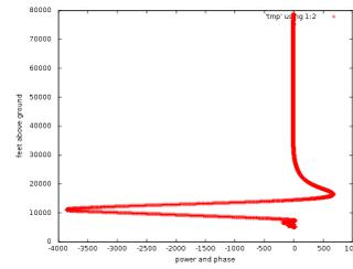
Figure 12: The output from the exponential chirp filter with 450 units of width and 600 ticks at 48MSPS in length for a chirp with RX delayed by 500 samples directed upward at 12dBi to a METAR stated cloud ceiling of 12000FT. See figure 17 in the figures section on page 12 for a full scale image.
