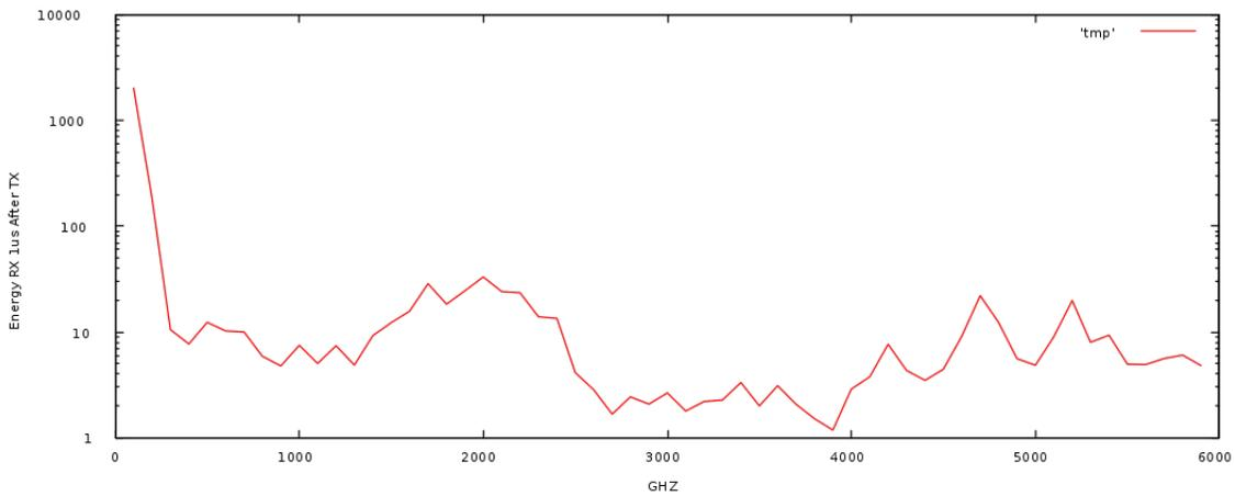
**Figure 16: The energy measured at the specific frequency after a 1024 samples at 6MSPS. The horn was directed upwards.**
