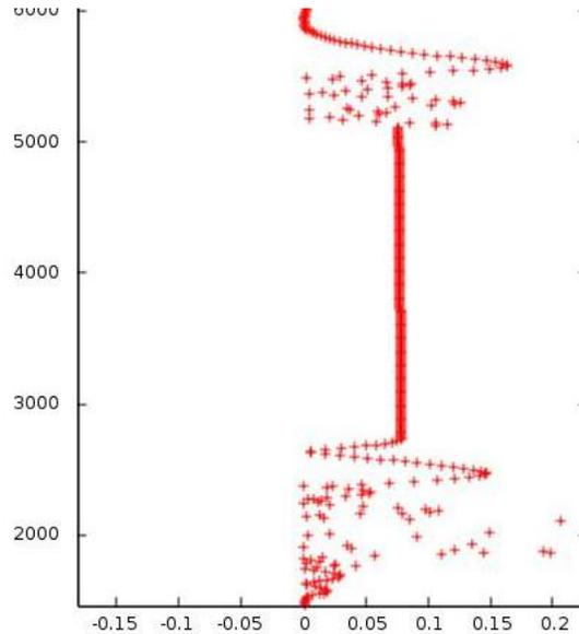
**Figure 15: A higher resolution cloud reflection which what may be a double reflection above (reflection from cloud to ground to cloud and back). The data correlates with weather reports of clouds base at the time.**
