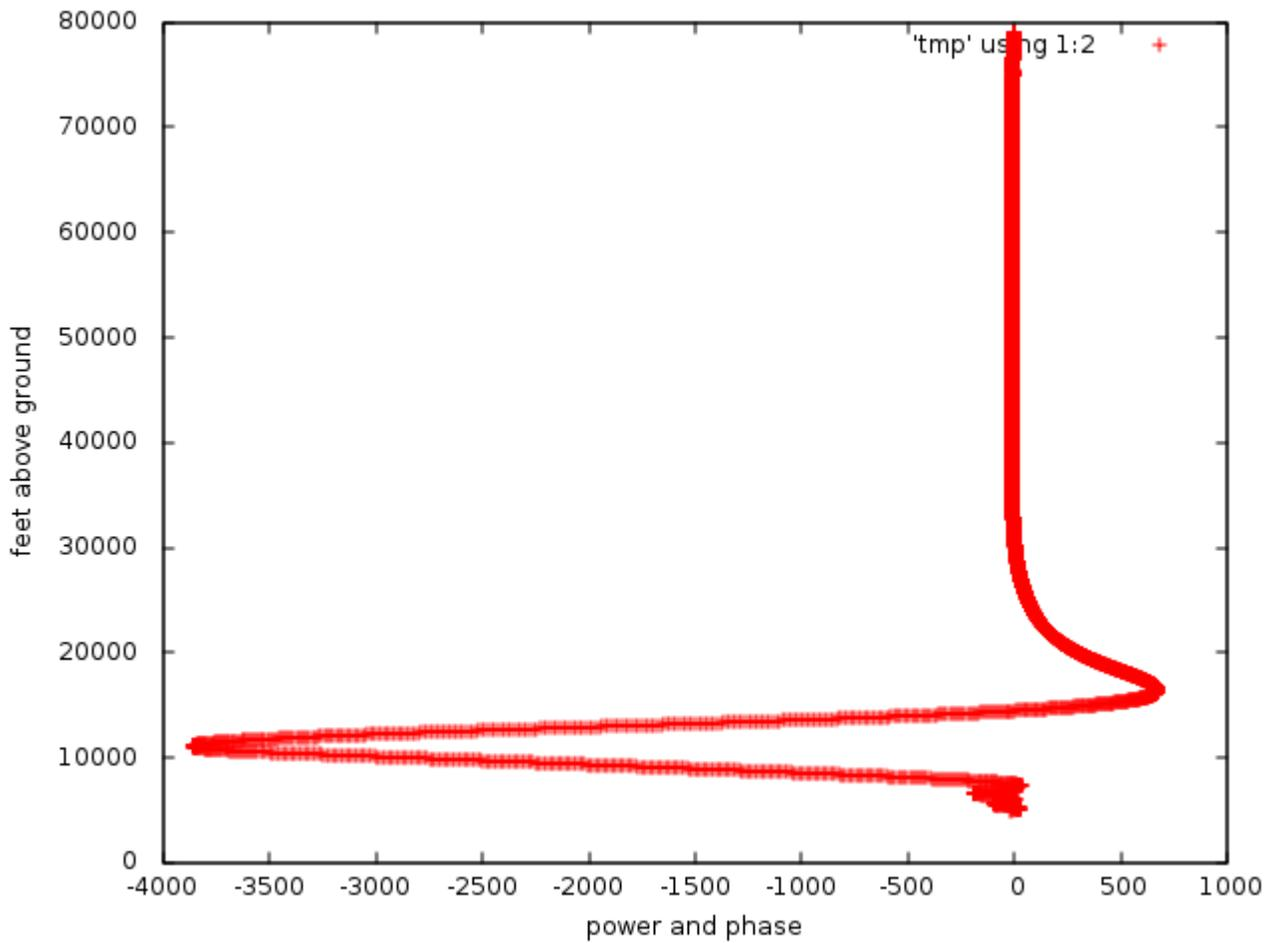
**Figure 17:** The output from the exponential chirp filter with 450 units of width and 600 ticks at 48MSPS in length for a chirp with RX delayed by 500 samples directed upward at 12dBi to a METAR stated cloud ceiling of 12000FT.
